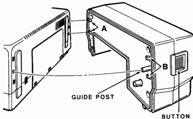
**Figure 1-7. Battery Installation**
