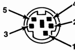
Figure 5-13. Numeric Keypad Connector
