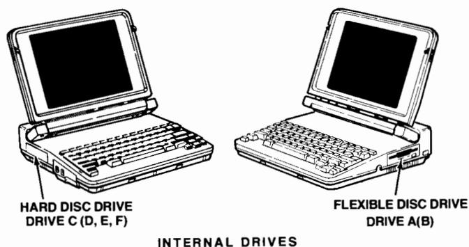
**Figure 5-1. Disc Drive Identification**
