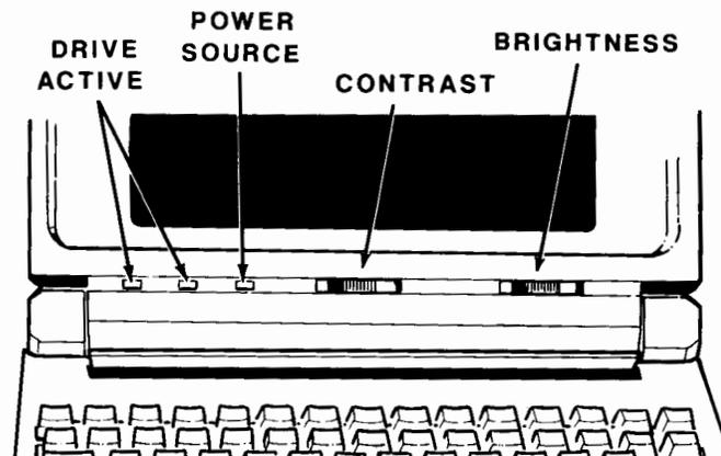
Figure 1-3. Brightness and Contrast Controls
