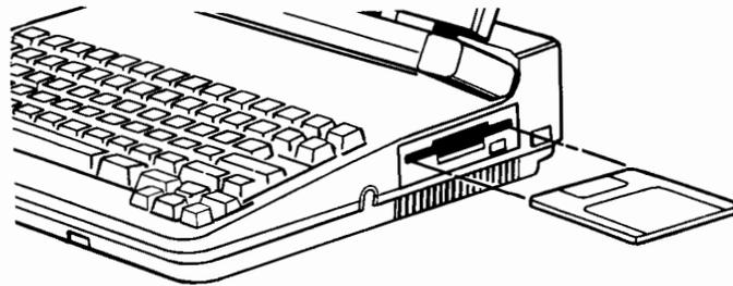
**Figure 1-4. Inserting the SETUP Program Disc**
