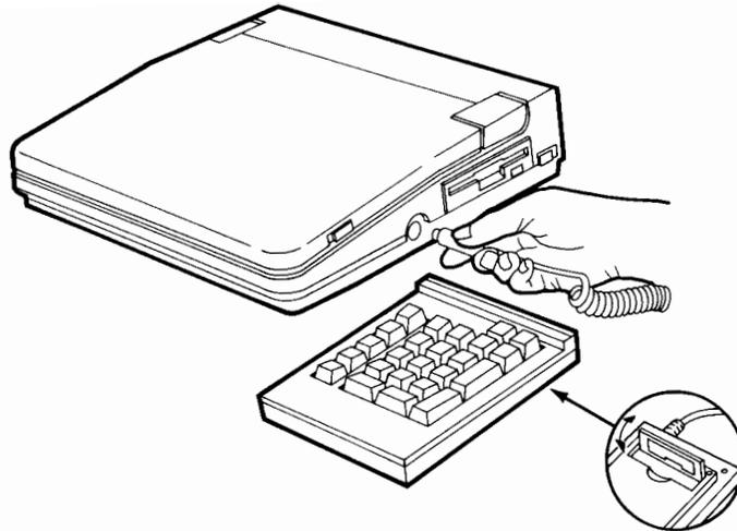
**Figure 2-4. Connecting the Numeric Keypad**
