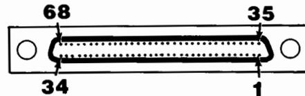
Figure 5-5. Expansion Chassis Connector
