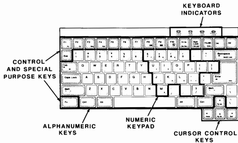
**Figure 4-1. Keyboard Arrangement**
