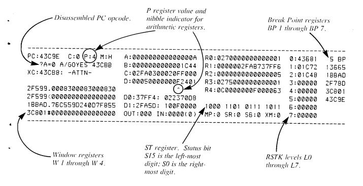
Figure 3. Debugger 80-Column Display
