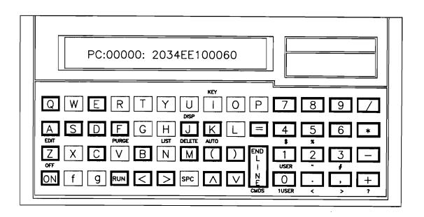
Figure 2. HP-71 Debugger Keyboard
