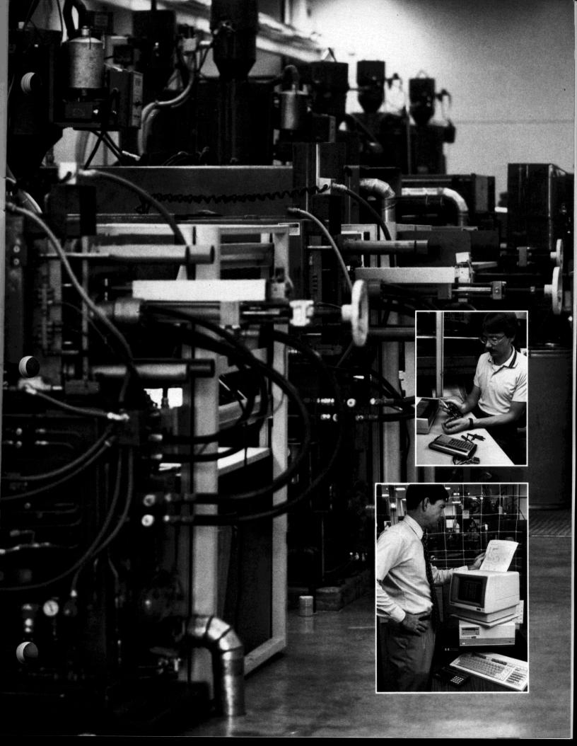
The machine operators also input part data by pressing HP-71 keys that have been redefined to represent each type of part defect tracked. And custom keyboard overlays are used so each operator can easily identify which key to press.
