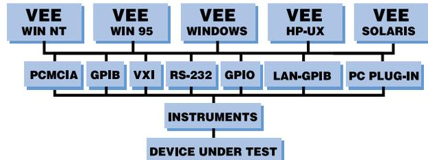
HP VEE can talk to a broad range of instruments through direct I/O, the 450 VEE drivers or any industry standard VXIplug&play driver!
