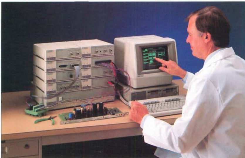
PC Instruments System Software converts a computer screen to a "soft front panel" that duplicates the front panel of a conventional instrument. To operate an instrument, you merely touch the screen.
