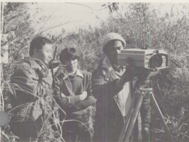
YHP civil engineers demonstrate the accuracy of the HP3808A range distance meter.
