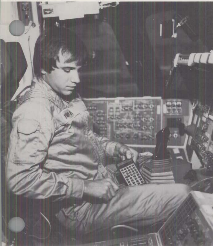
SPACE SHUTTLE. Two HP-41C calculators on board the Space Shuttle Columbia helped control its landing by monitoring the center of gravity and directing fuel use accordingly. The calculators also told astronauts John Young and Robert Crippen which communication stations were within reach throughout their flight.
