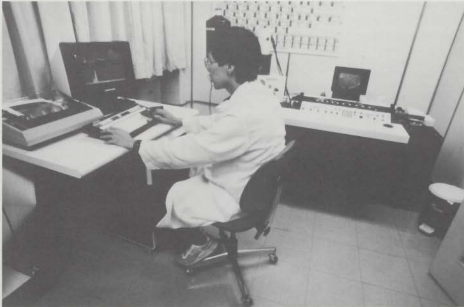
Sophisticated failure analysis equipment such as this SEM/EDX system help in troubleshooting.
