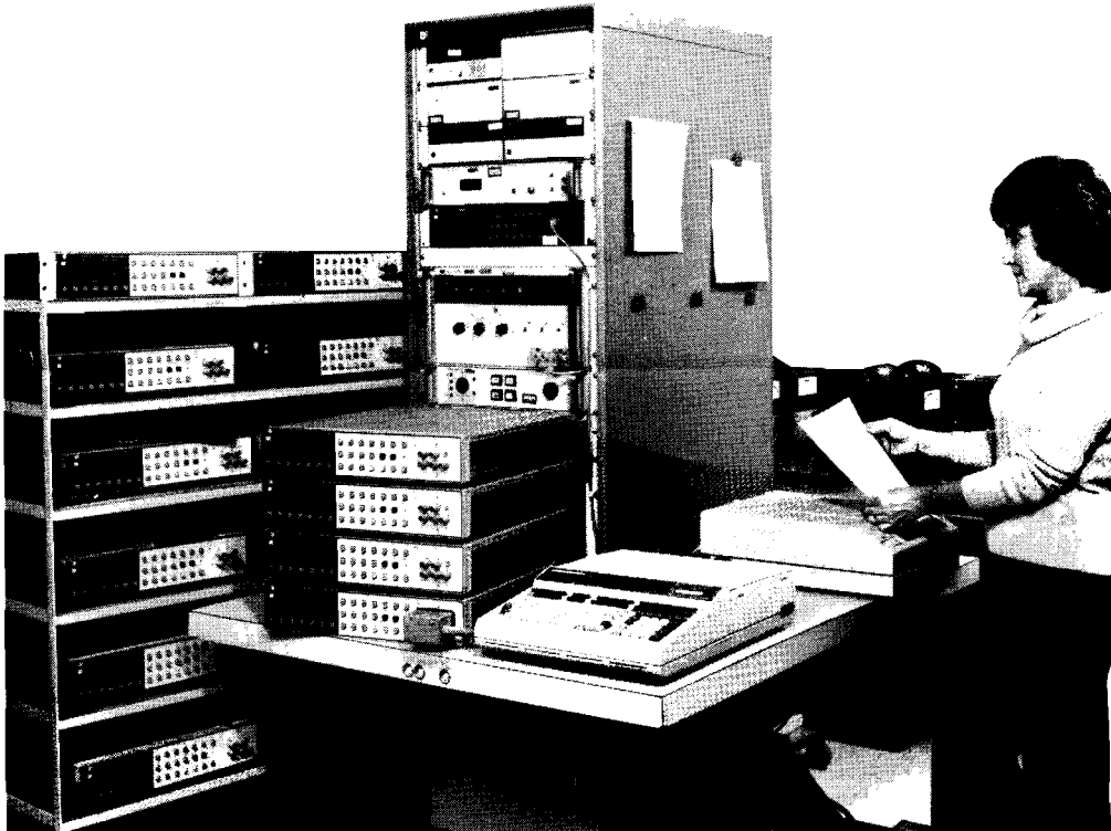
A 25T Desktop Computer controls the automated testing of digital voltmeters, acquires test data and prints out results on an HP 9876A Printer.
