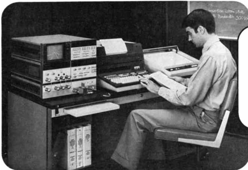
Response plot of Microwave Radio Link 70 MHz IF bandpass filter showing insertion loss and group delay vs frequency. HP 8505 permits simultaneous measurement of these parameters so that interactions of adjustments can be optimized for lowest distortion.
