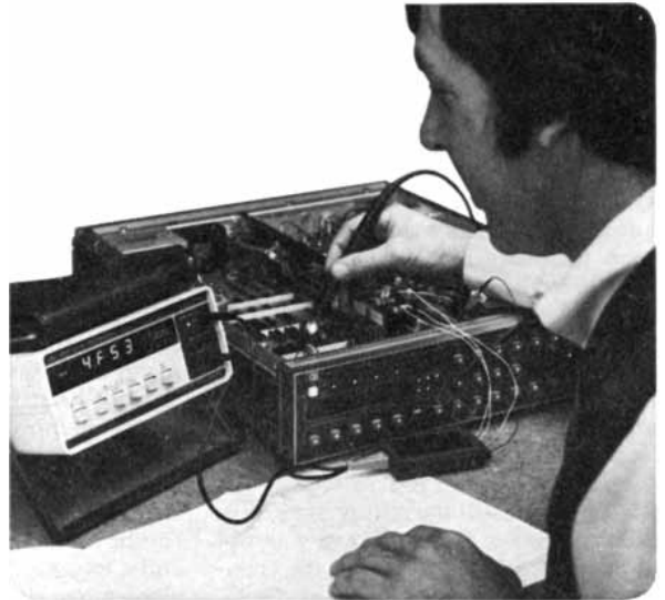
Four-digit signature displayed by the HP 5004 signature analyzer (the instrument to the left of the unit under test) greatly simplifies the identification and correction of faulty digital circuits at the component level.
