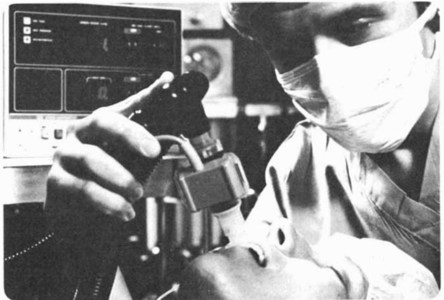
A beam of infrared light from the sensor is transmitted through the adapter, and the absorption of this light by the breathing gases gives an accurate, continuous measure of the patient's CO<sub>2</sub>.
