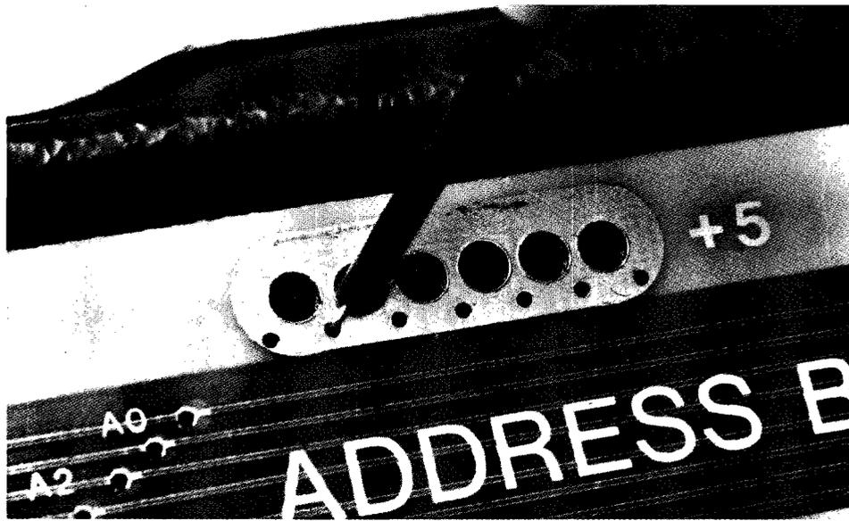
Figure 16-2. Using "Grabbers" to Get Power from  $\mu$ Lab's Power Slots
