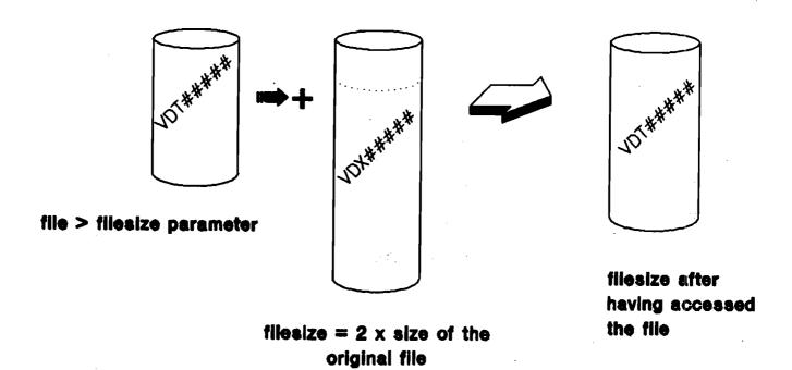
There are, however, applications that append data to an existing file. In such a case, PDSERVER creates a second file that is twice the size of the original file, regardless of which file size was configured for the shared disc. Again the files are merged, as soon as the writing process ends, to build a file whose EOF equals to the integer multiple of the 256 k file limit.
