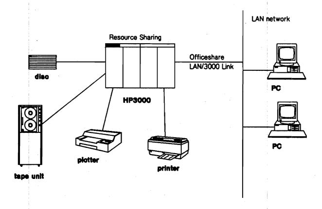
Resource Sharing is an HP 3000 software that allows PC users within a LAN network to use disc space and printers of an HP 3000. This means, on the one hand, that PC applications and data can be stored on one or more HP 3000 systems. On the other hand, several PC users may simultaneously use the different printers and plotters that are connected to an HP 3000.
