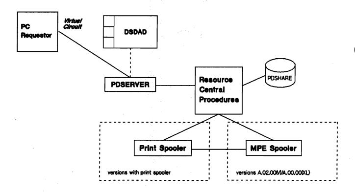
For every connection request a MS Net connection packet is sent via the virtual circuit to the PDSERVER. This packet contains the shortname of the shared disc or shared printer/plotter that is configured in the RESMGR. Now, PDSERVER invokes the Resource Central procedures to process the connection request. The file PDSHARE.PPC.SYS checks, whether the shortname is configured and whether the request refers to a disc or to a printer.
