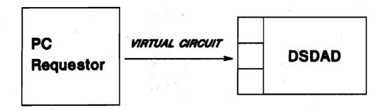
A connection request from a PC to an HP 3000 may be performed manually or automatically. If shared devices are configured in the AutousesMenu of the PC OfficeShare, the connection is set up automatically, as soon as the network is started. The connection may also be set up manually using the USE command (use device: \\servername\\shortname).
