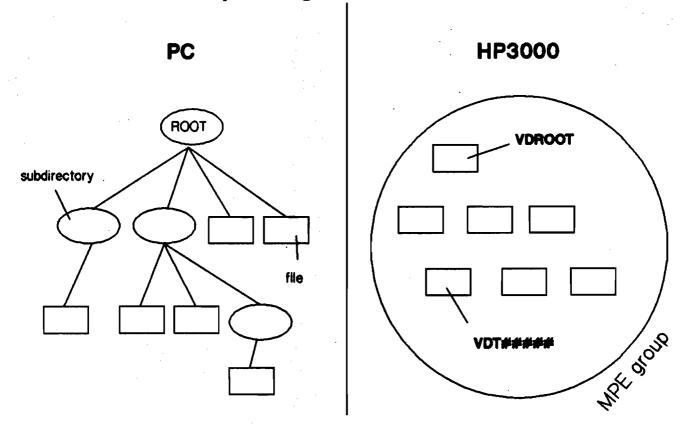
When creating a shared disc, an MPE file VDROOT is created in the desired group of the account. This file contains information on all files and directories that are kept on the shared disc and reflects the DOS file structure. The DOS files are represented by the VDT##### files on MPE level.
