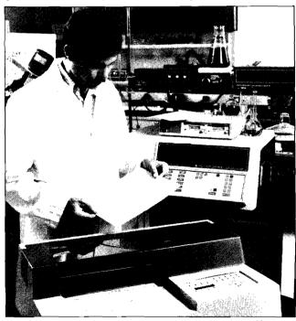
Because of its fast throughput and cut-sheet media feed, the HP 7550A is a good auxiliary B-size plotter for providing check plots and working copies of small sections of a larger plot. Also, because it is fast and operates unattended, the HP 7550A can be a shared central plotter for a number of workstations.
