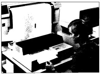
The new HP 7550A can be used as a central systems resource plotter in the computer room. It's ideally suited for this application because of its very high throughput and automatic cut-sheet paper feed.
