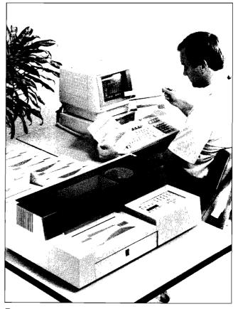
Fast, high quality duplication is now a reality using the new HP 7550A plotter. The "replot" function alows the HP 7550A to make up to 99 copies of a graph without rerunning the program.
