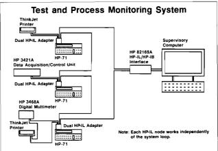
Plugging two HP-IL modules into the HP-71 is especially useful in manufacturing situations where control and com-
