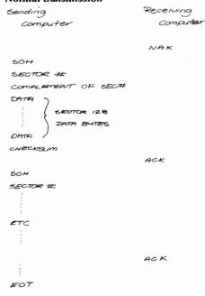
By definition, the receiving machine has to get into synch with the sender by first sending a NAK. The first sector is then transmitted and is re-transmitted if after a prescribed interval as ACK is not sent by the receiving computer, a certain number of re-tries is usually allowed before aborting the transmission.
