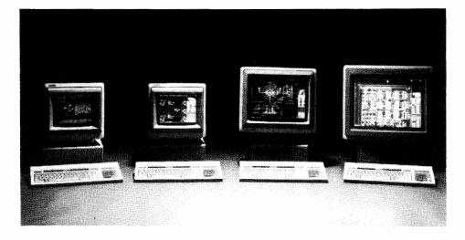
With the HP 9000 Series 300 users may pick from a 16/32-bit processor or a 32-bit processor, color or black and white, and medium or high resolution displays.
