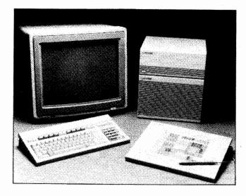
The HP 98700H Graphics Display Station consists of the graphic processor, a new 19-inch color monitor, and the HP-HIL keyboard (the digitizer tablet is optional). The HP 9000 Model 550, needed to run the system, is purchased separately.
