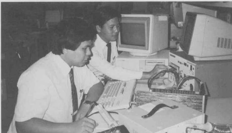
David Lim (foreground) and Dawson Ng use a test jig shipped from Sunnyvale to verify the operation of the reworked Vectra boards.
