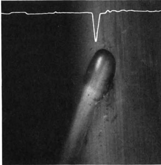
fectometer obviously has other applications than on the Texas range. It can locate faults in the maze of cables on aircraft, in buried cables, in cables on production lines, or in cable connectors. It operates up to 12.4 gigahertz ( $12.4 \times 10^9$  Hz). Reflectometer, sampler and step generator cost \$3150. If you need only inches of resolution rather than millimeters, a less expensive system sells for \$2125. Of course, you'll need the HP 180A Portable Oscilloscope, at \$825.
